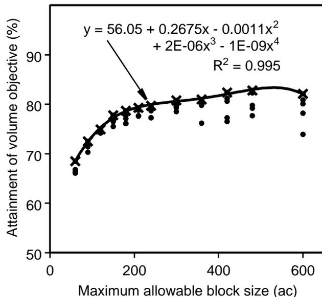
**Figure 6.** Effect of maximum allowable block size on attainment of 15 yr harvest volume objective. The trend line was developed by regression of the highest attainment values found.
